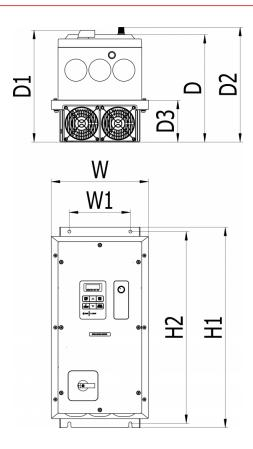
$\begin{array}{ll} D & = 246.6 \\ H1 & = 460 \\ W & = 222.8 \\ W1 & = 140 \\ Weight in (KG) = 12.68 \end{array}$
